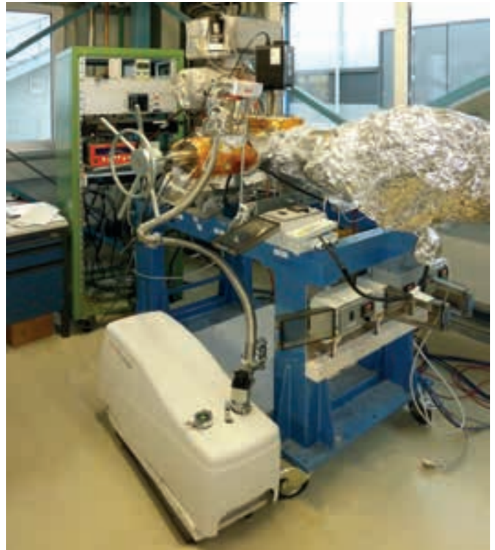
Figure 2: Test setup for qualifying a pump combination of ACP backing pump and HiPace turbopump
