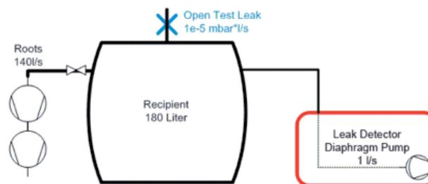
Figure 2: Steeper signal rise due to a parallel pumping station with high pumping speed
