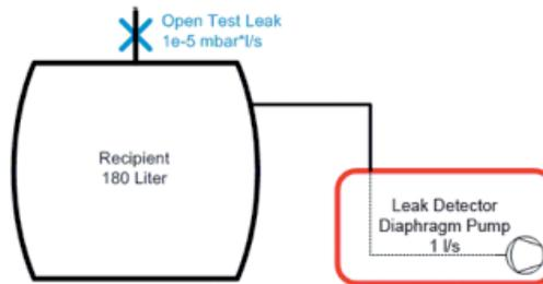
Figure 1: Slow signal rise with time delay due to low pumping speed
