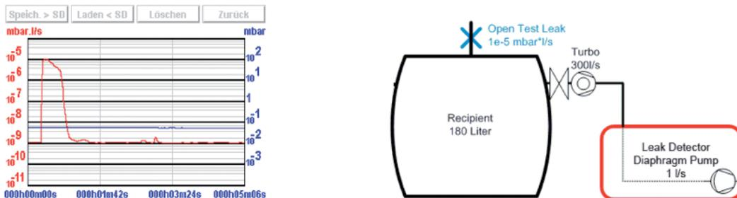
Figure 4: Signal response and decay behavior of a series connection of a high-vacuum pump and a leak detector.
