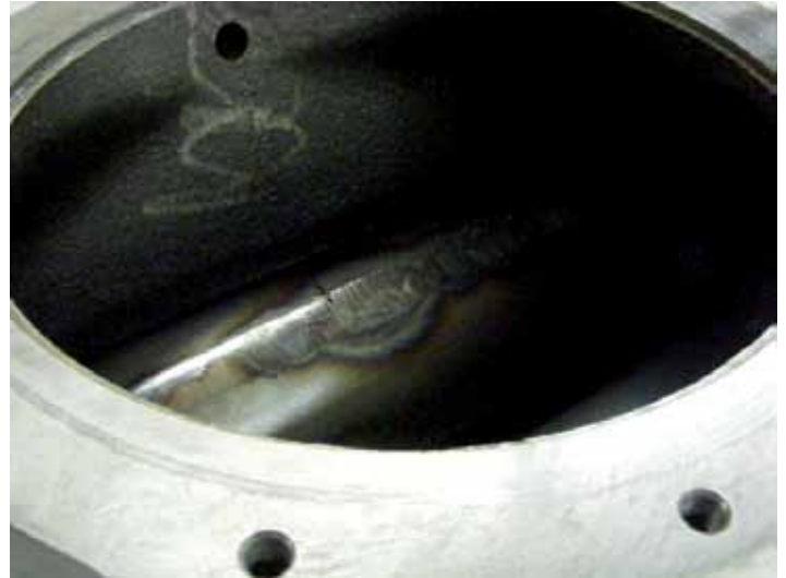
Figure 1 and 2: Roots pump seized by switching to ultimate pressure and the resulting local overheating
