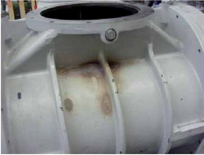
Figure 1 and 2: Roots pump seized by switching to ultimate pressure and the resulting local overheating
